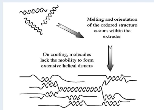
Figure 2. Model of xanthan gum molecular organisation resulting from extrusion and subsequent drying.
