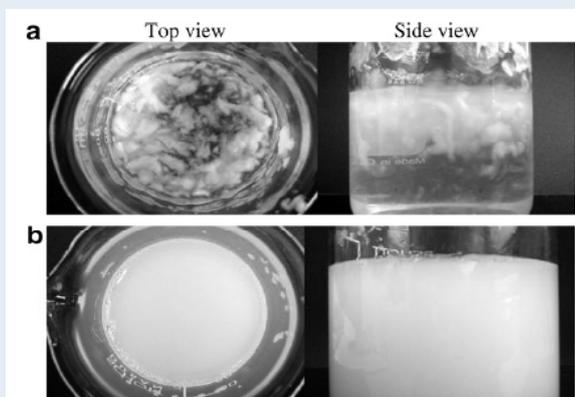
Figure 1. Xanthan gum dispersion in distilled water (0.75% wet weight basis): (a) non-processed xanthan gum and (b) extruded xanthan gum (dispersions prepared by mixing with a spoon for 10 s).
