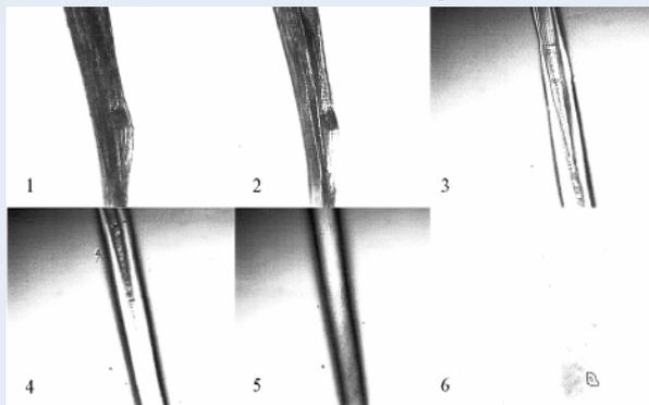
Figure 1. Microscopic images of bacterial cellulose (BC) Native BC (1), after contact with the ionic liquids (2), after 5 min (3), after 10 min (4), and after 15 min (5) and 20 min (6), K. Schlüter et al., *Macromol. Rapid Commun.* 27 (2006) 1670-1676
